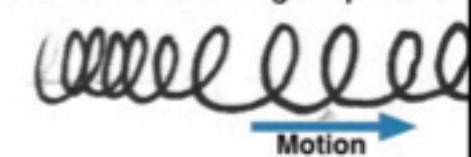
Diagram 2: Longitudinal waves move back and forth along the path of motion.
